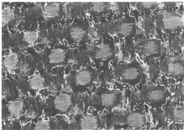
Figure 7 Optical micrograph showing a crack and a void near a resin-rich area.
